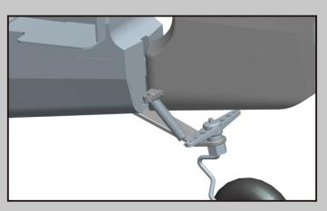
9. Connect the rudder linkage to the rudder control horn from bottom of the plane (Bolt:2.0x10 1pc, M2 nut: 1pc).
