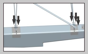
19. Install the floats to the fuselage using 2 strips and 2 spars (3.0x10 4pcs), connect the water rudder servo extension to Receiver.
