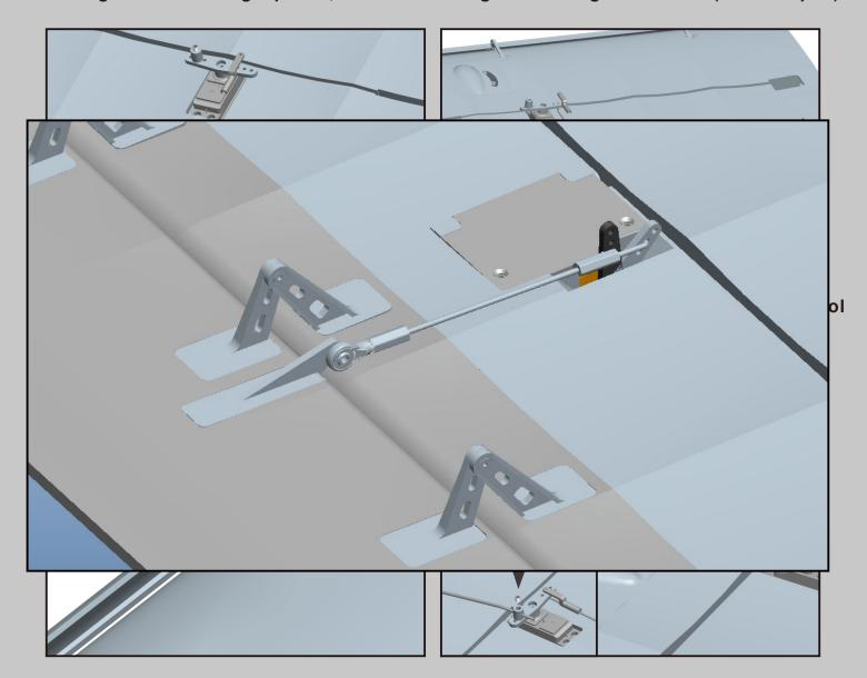
Optional slats: You can fix the slats by tape the T/E to the wing, so you do not have to install the rods and the linkage in this step.
