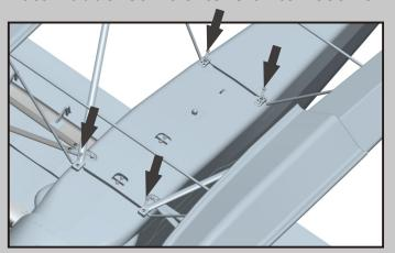
20. Install the wing fences and LEDs.
