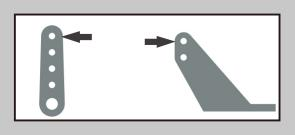
12. Try assemble the wing struts make sure the axile of the mounting plastics align well(A). Secure with the provided screws with the Struts(B),
