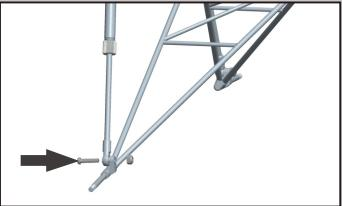
5. Install the mounting plates to each sides of the fuselage (2.6x12 4pcs). Bolt the landing gear assembly to the fuselage (3.0x14 4pcs).
