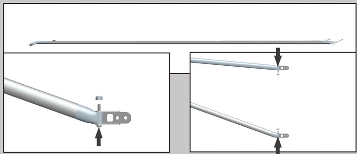
14. Try Install the wing struts assembly to the wing as the picture show or you have to change to the other one.(2.3X10 8PCS)
