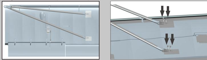
15. Insert the main spars into place, the shorter one in front (10x8x450mm 10x8x600mm), install the main wing into place until the mounting nuts on the wing root aligned perfectly with the holes on the mounting pocket. Secure the wing with provided bolts (3.0x8 4pcs).
