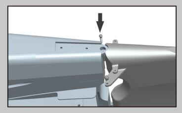
8. Install the tail wheel assembly into place and fix it with provided screws(2.3x12 2pcs), Connect the rudder to the steering arm.
