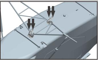
6. Bolt the Absorption rods to the gear mounting plates (Bolt: 3.0x14 2pcs, M3 nut: 2pcs), install the wheel assembly to the wheel shaft. (M4 nut: 2pcs, come with the Gear SET).
