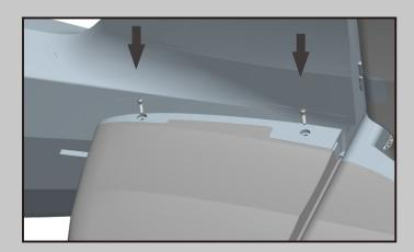
11. Connect the Elevator linkage to the Elevator control horn from tip side of the stab (Bolt:2.0x10 1pc, M2 nut: 1pc).
