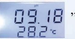
meter enter the pH9.18 automatic calibration mode. While display value correspond to the standard buffer solution, the calibration is finished. Users can choose the calibration solution 6.86 4.00 9.18, 7.00 4.00 10.00. Factory default calibration is 6.86 4.00 9.19. The operation is
