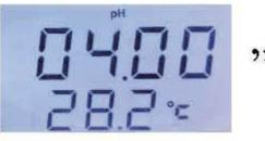
meter enter the pH4.01 automatic calibration mode. While display value correspond to the standard buffer solution, the calibration is finished.
